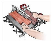
**Adjustable Guards** are barriers that adjust for a variety of production operations. These adjustments are made by the operator depending on the size of the materials the operator is working with. If these guards are adjusted properly they will protect you, if not adjusted properly they will not!
