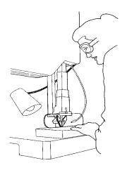
Interlocking Guards work in the same way as Fixed Guards but are often used to guard parts that may need to be accessible during tool changes or jams. When the guard is removed the machinery shuts down and cannot restart until the guard is replaced.
